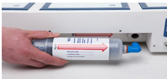
Figure 12.2 The way of pulling filter
